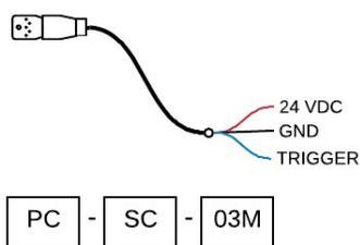
The power cable is used to power the dual output junction box (PN JB-DU-AM-1C). Typically terminated through a cable gland into an existing electrical cabinet. Comes standard with **3m** length.
