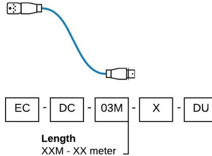
Extension cables can be used to increase the length of existing cables. Available in: **3m, 10m** lengths
