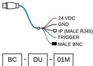
Breakout cable providing access to the internal connections of the ToughEye. Typically terminated through a cable gland into an existing electrical cabinet. Comes standard with **1m** length.
