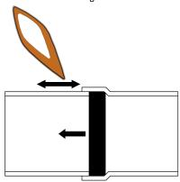
5) Begin brazing by concentrating heat on the male side of tubing, transitioning to applying heat all around the joint.
