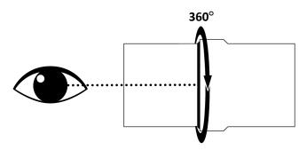
6) Braze is completed when molten braze alloy becomes visible around the full circumference of the joint.
