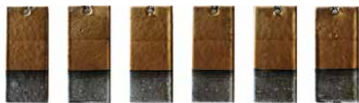
Figure 2, Coating 1 panels, post-autoclave.
