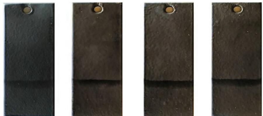
Fig. 5: Coating 2 panels, post autoclave test. (Left to right): 2A, 1B, 2B and 1C.
