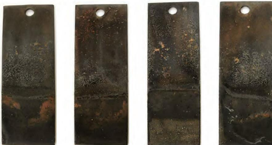
Fig. 2: Examples of deliberately contaminated panels.
