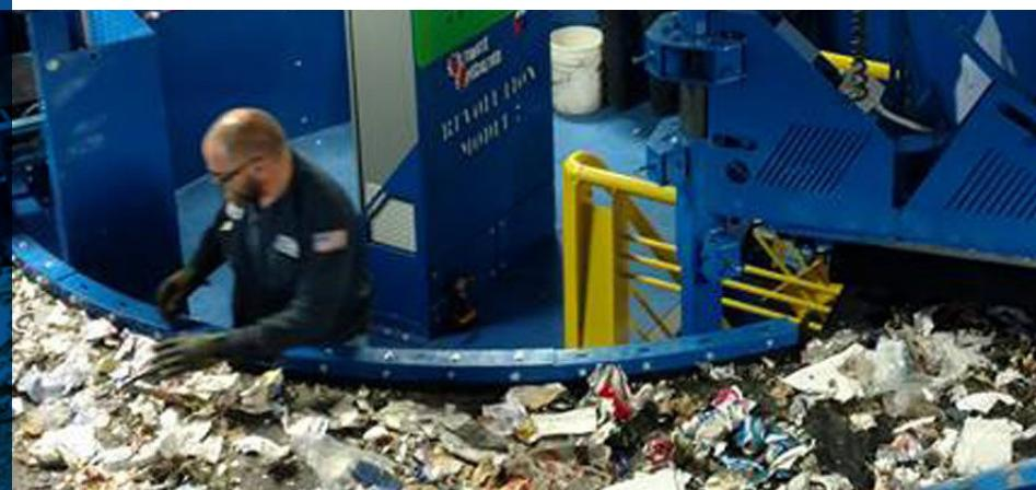
Revolution Systems' patented recycling machine and process consists of a circular system called Revolution that enables the sorting of recyclable material by type, such as glass, plastic, and paper. The sorted refuse is then compacted into bundles, weighed, and sold to processors for conversion to new material. In 2020, Revolution Systems turned to StratusWorX and its leading Cloud Workspace technology to further streamline its game-changing recycling process.
