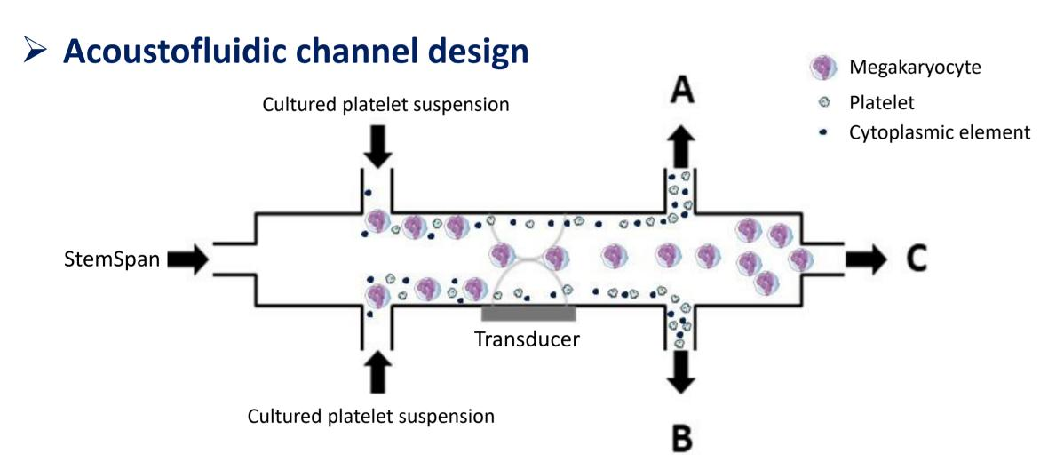
At this first step of procedure, platelet suspension is injected into the lateral inlets while StemSpan is injected in the central channel. Each inlet and outlet is driven at 0,5ml/min. An acoustic wave at 1,85MHz is applied to displace cells toward the C outlet.
