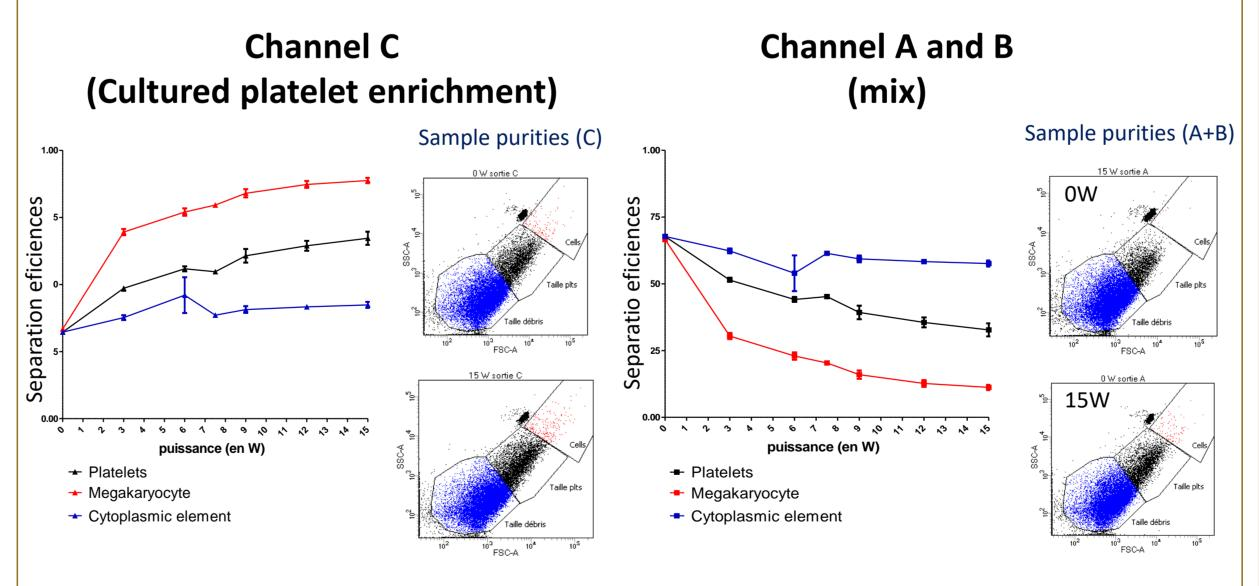
The optimal cultured platelets separation is obtained at an acoustic power of 15 W.
