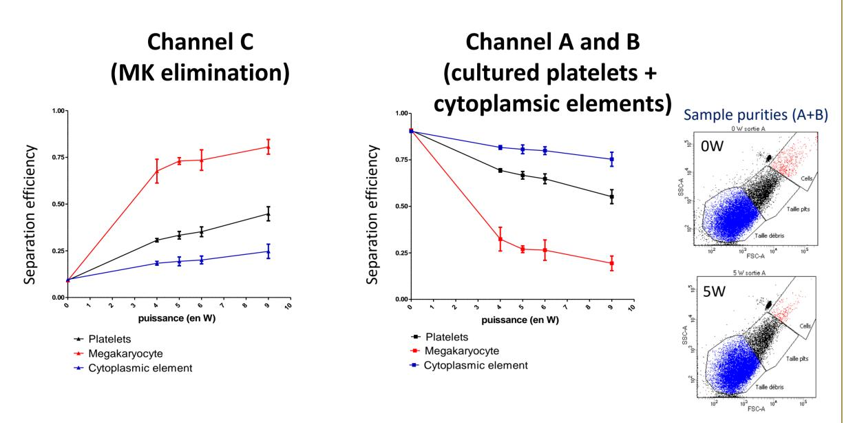
The optimal platelet suspension fractionation by acoustophoresis is obtained at an acoustic power of 5W.
