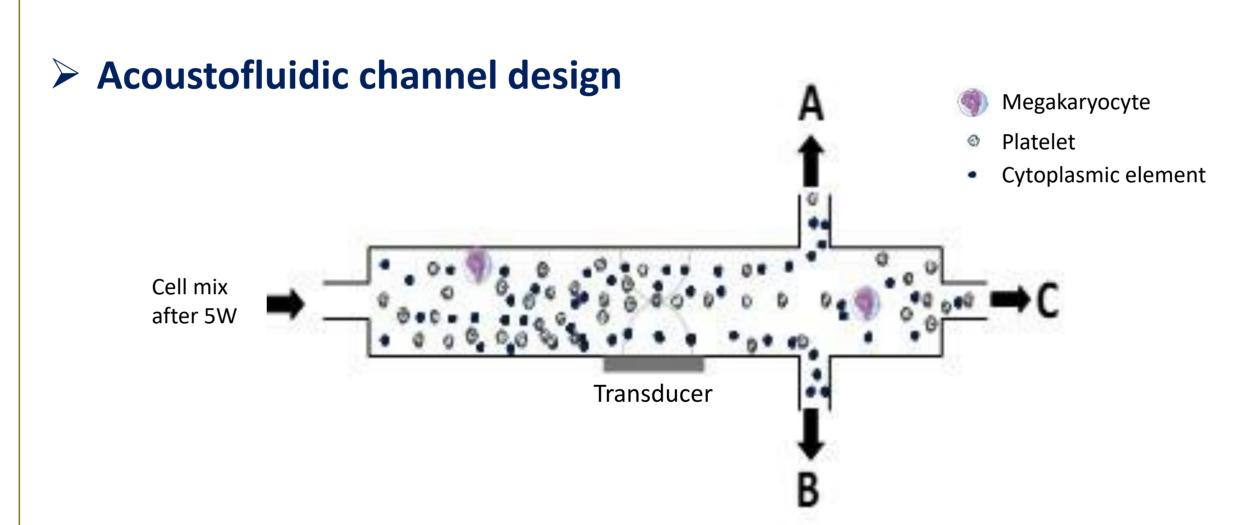
At this second step of purification, the cultured platelet suspension treated for MK elimination is injected into the focusing channel. The acoustic wave frequency and outlets flow rates are identical to the previous step. The inlet is driven at 1,5ml/min (3x0,5ml/min).
