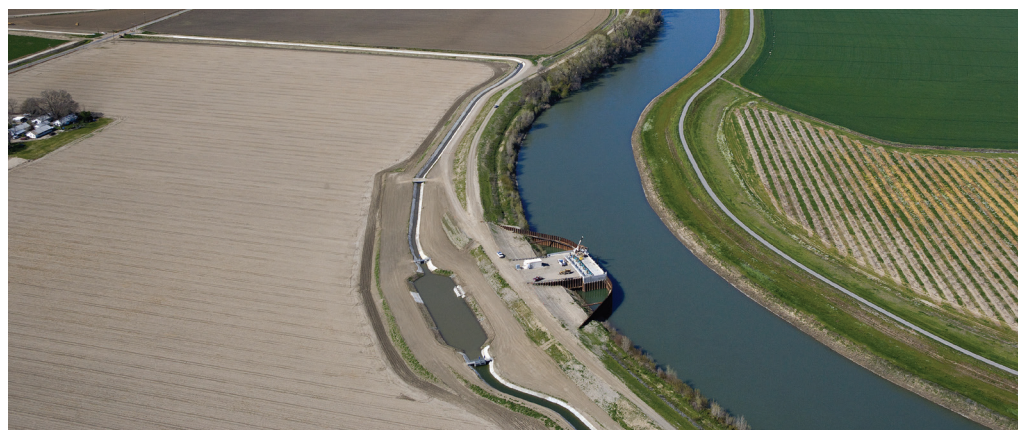
An aerial view showing the new pumping plant drawing water from the Sacramento River into the afterbay, which feeds the North and South channels.
