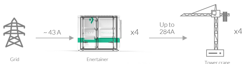
Figure 1. 'Block' diagram of the connection between the utility, Enertainer and the loads.
