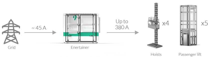
Figure 1. 'Block' diagram of the connection between the utility, Enertainer and the loads.
