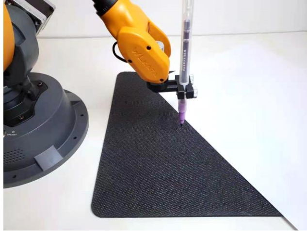
Figure 3.35 Placing a thin soft cushion under the paper to provide buffering during drawing
