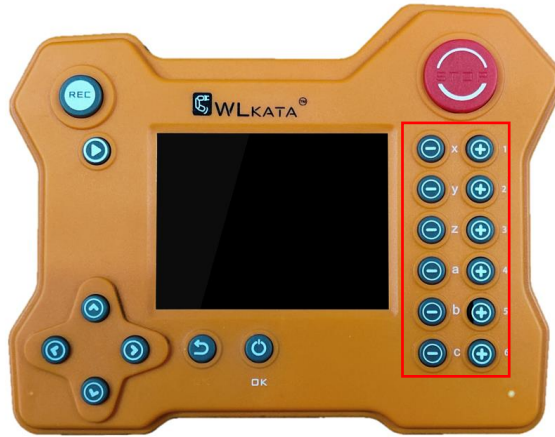
Figure 3.55 The 6 groups of buttons converted to control the end position and orientation
