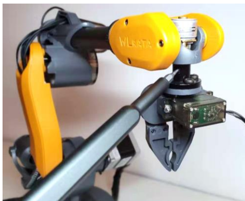
Figure 3.28 Installing the gripper module by a hex screwdriver
