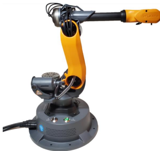
Figure 3.14 The correct manipulator position after a successful HOMING action
