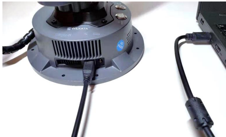
Figure 3.2 Connecting the manipulator to the computer
