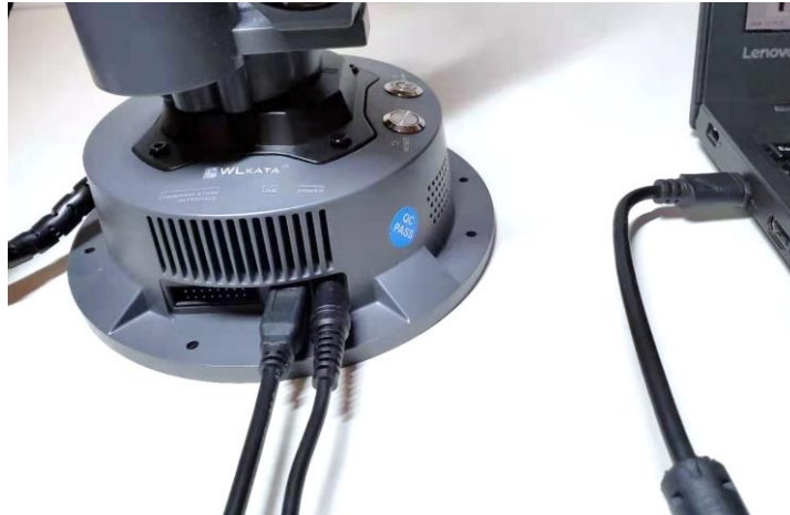
Figure 3.3 Connecting the manipulator to the power adapter
