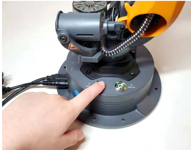
Figure 3.16 Pressing RESET button on the base of the manipulator after a software emergency stop
