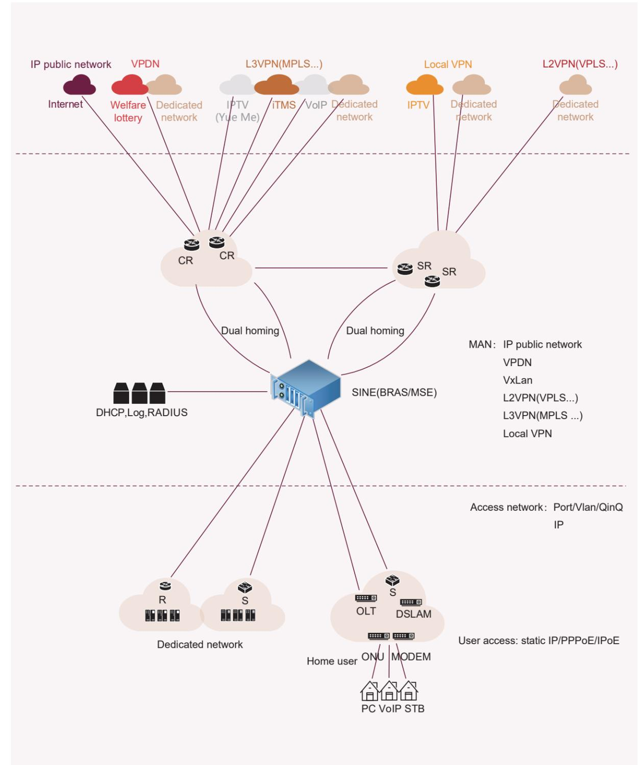
After authentication, authorization, and successful connection through PPPoE, the home broadband user's private address is converted to a public network address on SINE before the user can access the Internet, as shown below:
