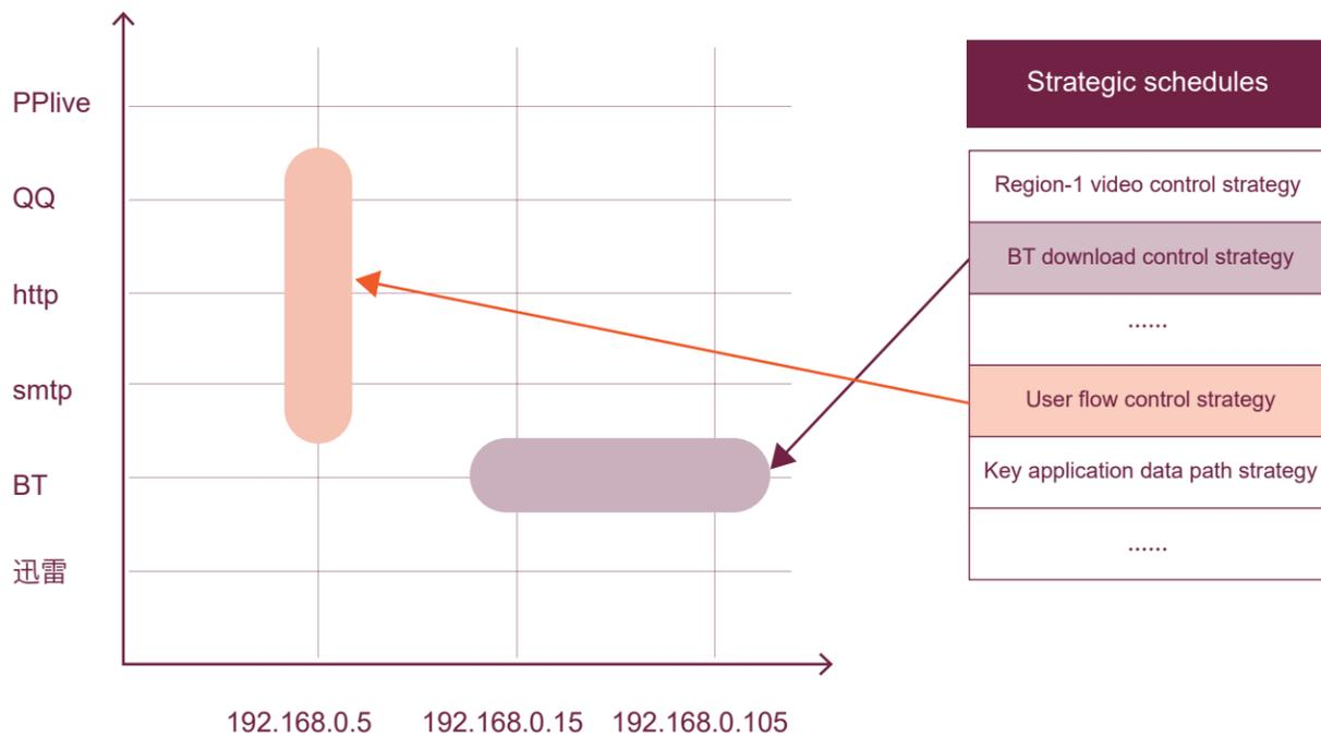
Diagram 3: SINE optimizes the caching queue, divides the original simple single queue into multiple priorities of the same type. High bandwidth applications such as webpage loading, real-time application, video, and online games are set to the high-priority queue. Network data received by SINE are processed according to their queue priority.
