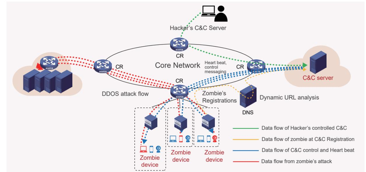
By taking advantage of large scale deployment at all the key gateway links in the network, SINE can integrate any DDoS detection subsystem (our own or any 3rd party) to achieve DDoS near-source suppression. It will not only reduce network resources earlier but also improve the resilience against any attack. The specific implementation method is as follows:
