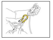
The ROLLCLIP Z pulley can be used for tree care to attach the ZIGZAG descender to the attachment bridge on the SEQUOIA harness, for improved lateral mobility.
