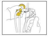
The ROLLCLIP Z pulley may be used as a directional point on the upper attachment point of the ASCENSION handled rope clamp, for short rope ascents. Gate opening on the non-pulley side facilitates installation on the ASCENSION.
