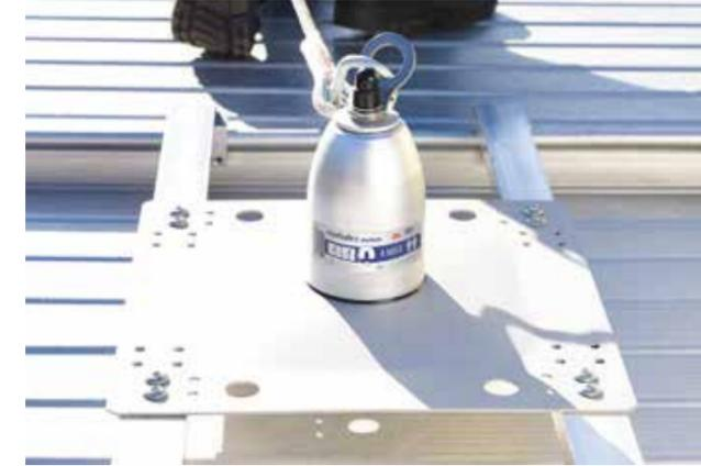
The RoofSafe Anchor from 3M™ Fall Protection has been designed to eliminate or substantially reduce the risk of injury or death to operatives working at height, whilst ensuring the integrity of the structure to which it is attached. The innovative 3M™ DBI-SALA® SpiralTech™ Energy Absorber results in the lowest forces back to the roof on the market measured at less than 6 kN.
