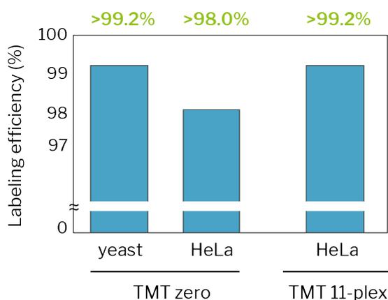
**Fig. 10** | TMT labeling efficiency for yeast and HeLa samples, 50 µg protein input. Lysis, digestion, TMTzero or TMT 11-plex labeling and peptide cleanup all performed on the PreON instrument.
