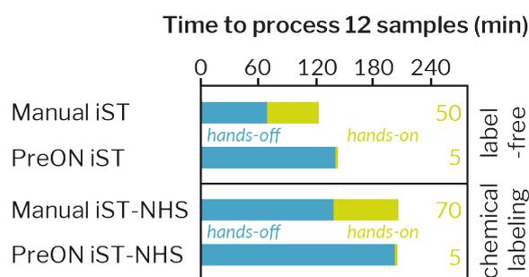
**Fig. 11** | Comparison of hands-on and hands-off times for a manual operator vs. operation on the PreON instrument. Top chart for label-free applications, bottom chart for chemical labeling.
