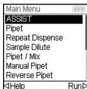
Select the ASSIST mode in the Main Menu of the VIAFLO pipette and press **OK**. The pipette establishes the connection via ComModul.
