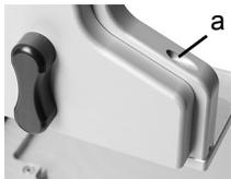
For fine adjustment of the pipette tips along the Y-axis turn the screw on the pipette holder (a) with a flathead screw driver size 2. Turning clockwise moves the pipette to the rear, counterclockwise to the front. The maximum Y-shift is +/- 5 mm.
