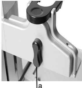
Set the lever (a) to the center to pipette in 96 well plates.
