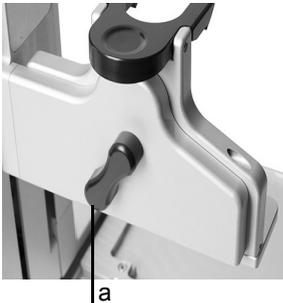
The rear position of the lever (a) moves the pipette to the rear to accommodate the rear positions of 384 well plates.
