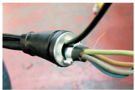
Thread encoder cable through motor power grommet
