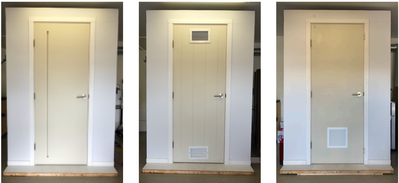
Figure 8 - Test Samples: VanAir Door, Two 6x10" Door Grilles, 10x10" Door Grille
