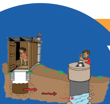
Latrines close to wells lead to contaminated water
