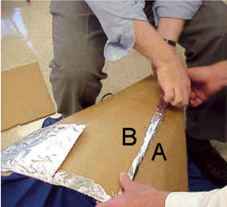
The easiest way to do this is to punch three holes in the cardboard that line up on side A and side B (see figure). Then put a metal brad through each hole and fasten by pulling apart the metal tines. Or you can use a nut-and-bolt to secure the two sides (A & B) together.
