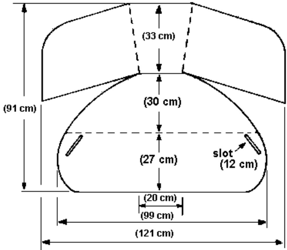
To set up, lay panel flat with shiny side up. Fold up front and back parts and fit back corners into the slots in front.
