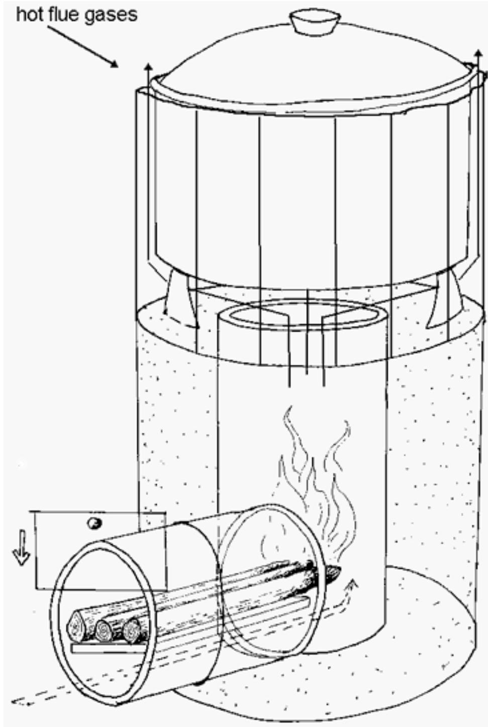
**This picture shows a thin piece of metal (a skirt) wrapped around the pot. This skirt forces the hot flue gases to rub against the bottom and the sides of the pots. The gap between the pot and the skirt should be about 1cm (assuming you are using an average-sized pot). In our tests, this simple heat exchanger (an old coffee can works well!) almost doubles the efficiency of the rocket stove.**
