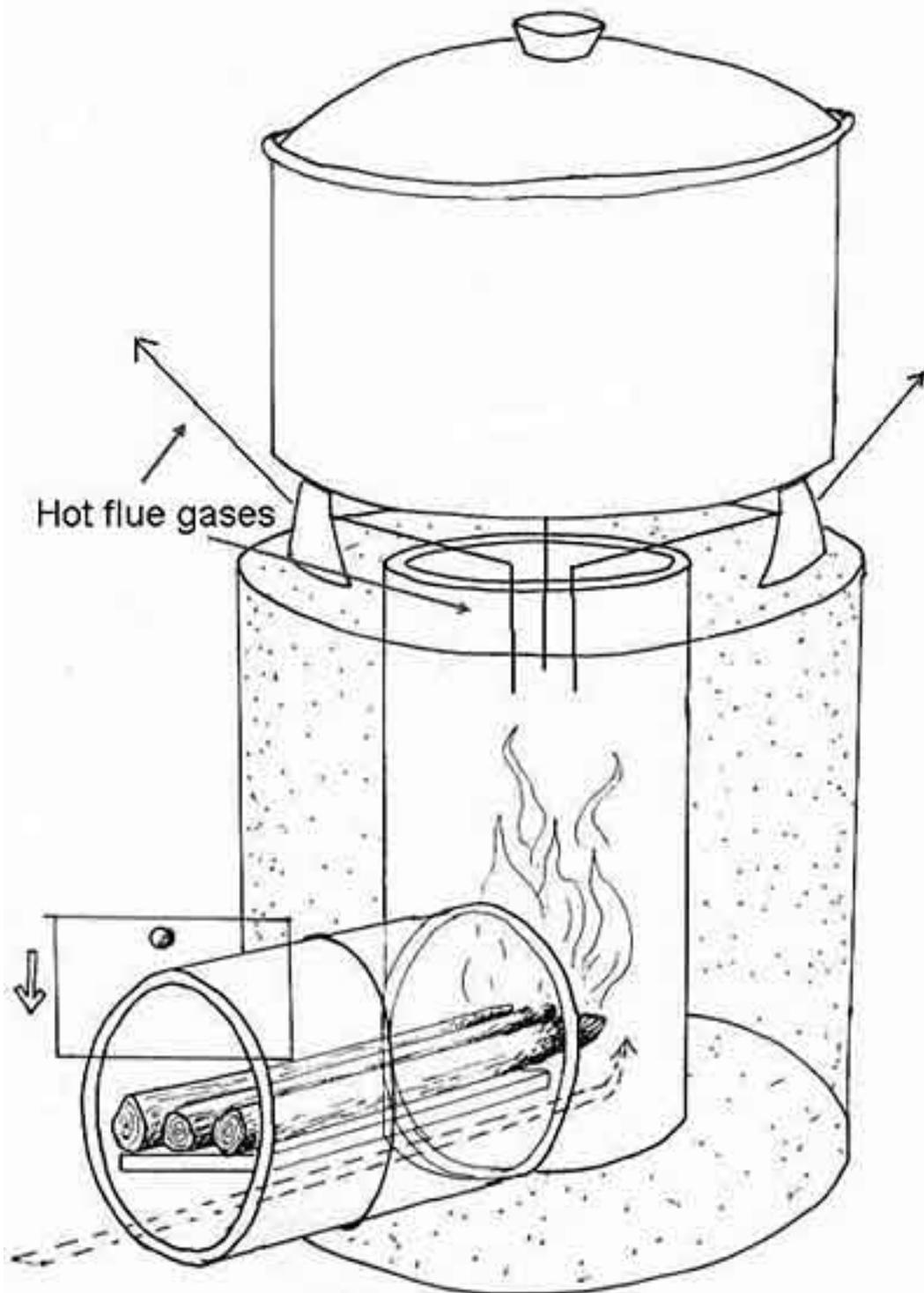
**This elbow is then placed inside of a container that is filled with insulation . The container can be made from almost any material. We have used 5 gallon drums, brick, clay, cement. For insulation we suggest using wood ash or perlite, or pumice,. Do not use massive things such as earth, sand, or cement. These will rob heat from the stove and reduce your combustion efficiency. For optimal use we recommend a 9" chimney and a 4" fuel feed magazine.**
