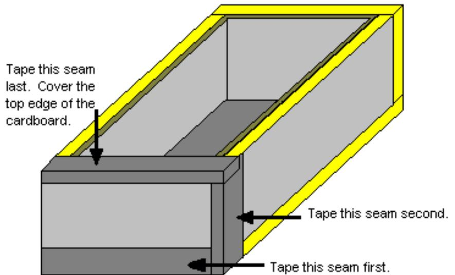
Figure 9. Tape the sheathing in place with aluminum foil tape.
