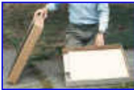
The lid fits perfectly onto the base of the larger box, so that, when collapsed, the cooker takes the form of a convenient, briefcase-size box.
