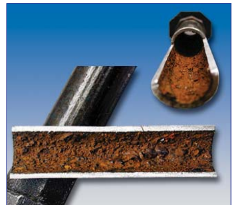
This actual cutaway of black iron compressed air piping shows typical contaminant build up and flow restriction after just a few years of operation.
