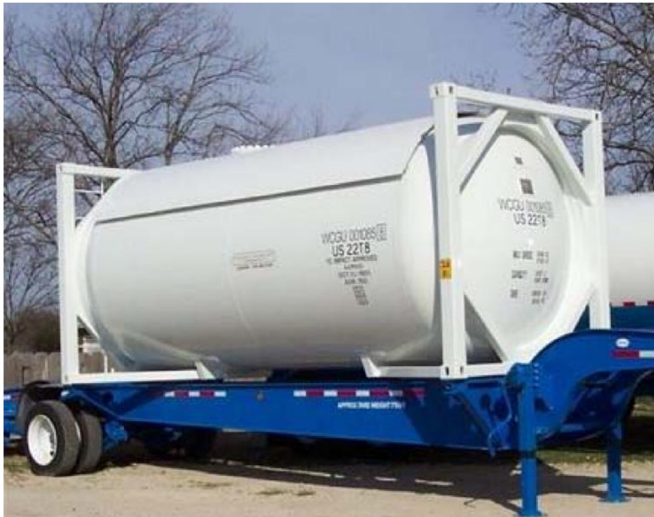
Figure C-4—Portable tank for liquefied gas (20 ft non-insulated tank container with sunshield)
