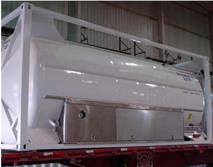
Figure C-1—Portable tank for refrigerated liquefied gas (20 ft cryogenic vacuum insulated tank container)
