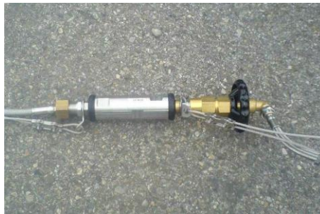
Figure 2 Typical breakaway coupling for gaseous filling
