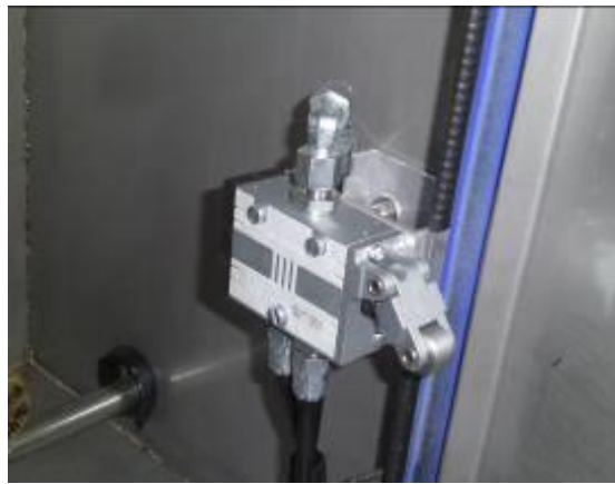
Figure B-2: Interlock with braking system active when cabinet door is opened
