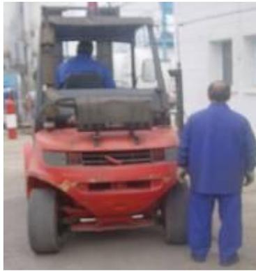
Figure 6 FLT reversing into path of a pedestrian
