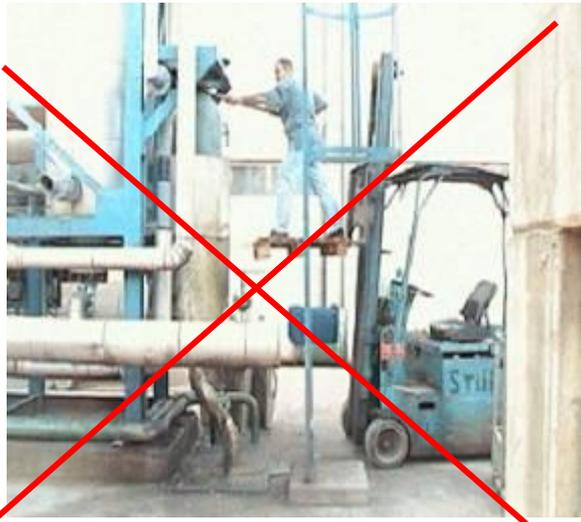
Figure 4: an unsafe use of an FLT
