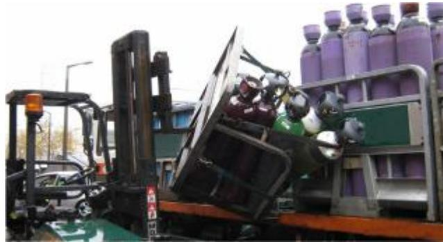
Figure 11 result of handling incident
