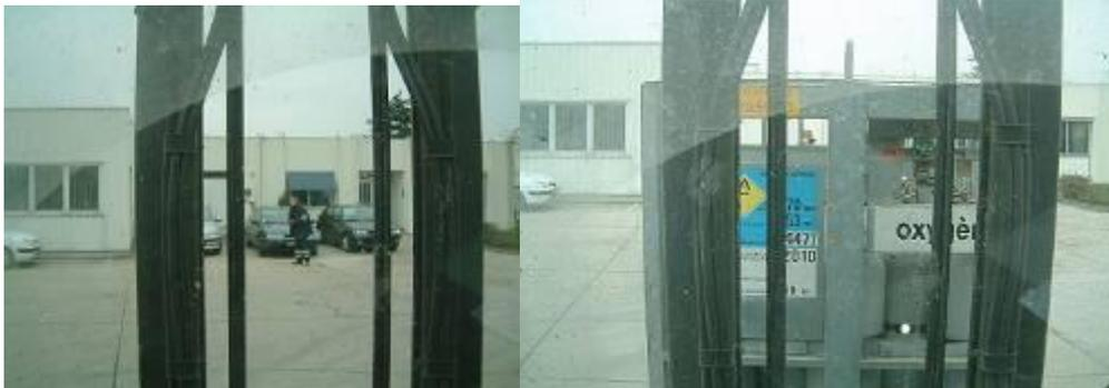
Figure 14: poor visibility when carrying cylinders pallets or bundles
