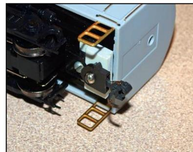
For the front coupler, the second piece – the one that is glued to the one you've already cut – is 5/8” side and 11/64” long. To see if it worked, I filed off the convex boss on the front cast
