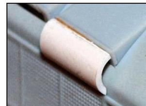
on how to get the most reliable service from their Babyface units, routed the heated air from the dynamic brake grids into the carbody and out through the top of the rear air intake screens. If No. 75 is the unit you're modeling, all you need to do is to take some 7/32" diameter styrene tubing (Evergreen No. 227), split it as shown in the accompanying photo, close off the ends with some sheet styrene, and glue them all in place.
