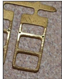
6. Two of the "straight" steps on the A unit and four of them on the B unit need holes drilled in them for the hand rails beside the engine room doors. These holes are located in the web between the top step and the vertical members and are drilled with a No. 77 bit.
