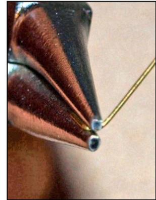
With all of the hand rails, you may have to tweak the bends to get the ends to properly line up with their mounting holes. But remember, sometimes it's easier to throw a hand rail away and make another one than spend a lot of time trying to adjust one that isn't "just right."
