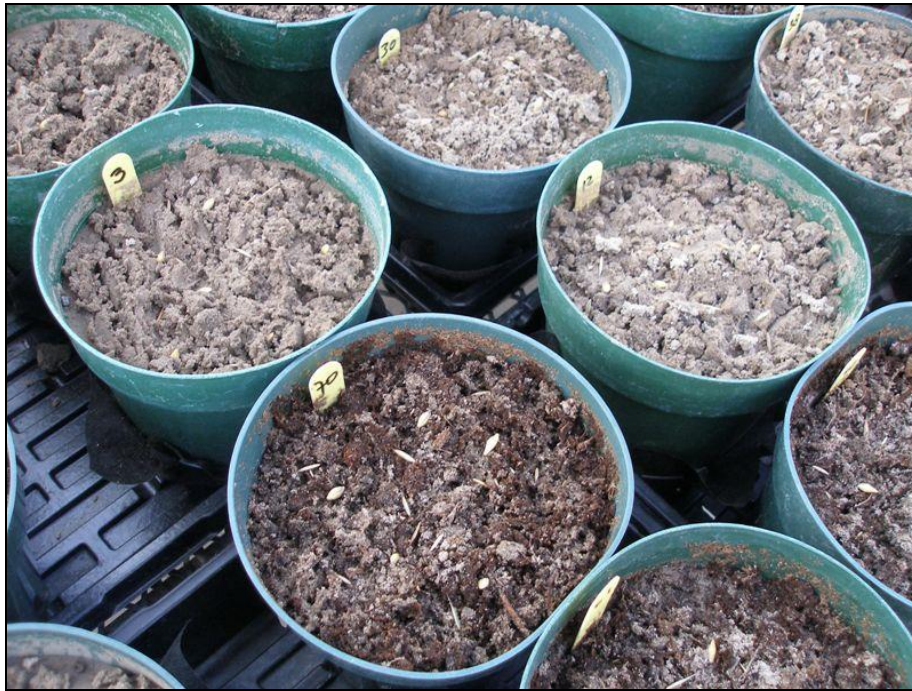
Figure 1. Tailings sand and tailings sand with peat amended with OM Plus and seeded in the greenhouse. OM Plus was evenly incorporated with TS (lighter colour material) and TSP (darker colour) before placement in the greenhouse.
