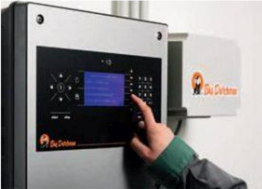
The station computer has a clearly arranged display and shows important information such as the status of the sow, the daily ration, the remaining feed quantity or the number of sows which have already eaten. It operates independently from the central PC for a high functional reliability. Sows that require special attention are identified by the control system and automatically selected. The farm manager is the one to define when and why a sow needs special attention.
