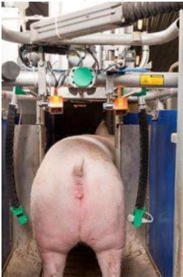
The station can also easily be opened in case of an emergency – thanks to the swing-type side walls.
