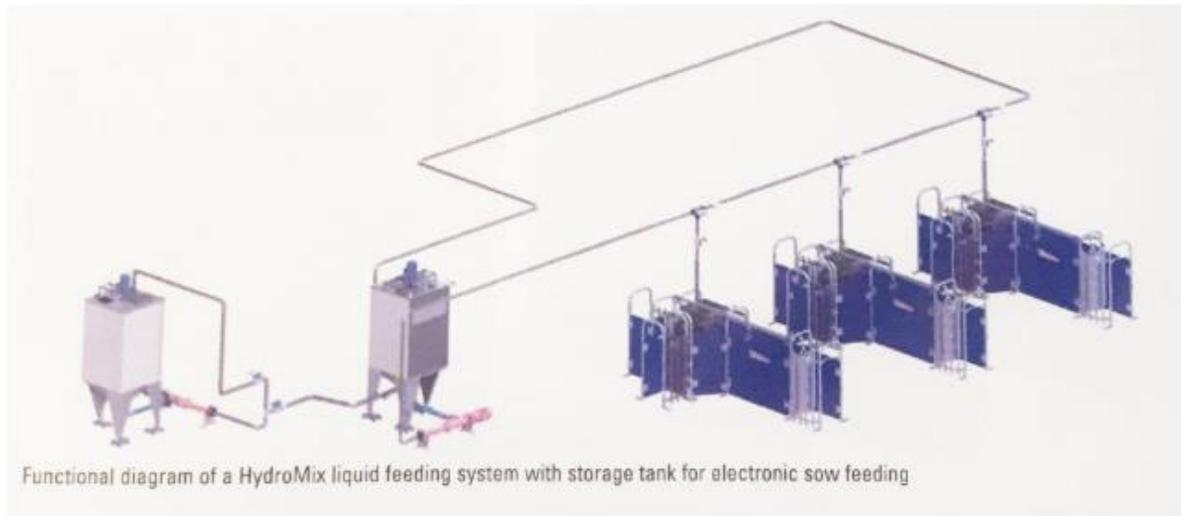
The exact amount of dispensed feed is determined by weighing the feed in the mix tank. If the stored feed mix drops below a certain minimum, the liquid feeding system receives a new request for feed. Moreover, the tank of the electronic sow feeding system returns feed which has not been consumed to the main system's mixing tank. This ensures that the feed remains fresh and increases hygiene.
