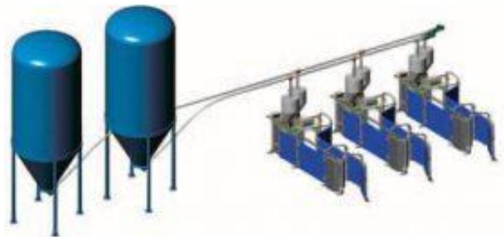
Each feeding station is equipped with a feed hopper supplied by the feed bin. A sensor in one of the hoppers supplying a group of stations registers when the feed level drops below a set minimum value. All feed hoppers are then immediately filled again.
