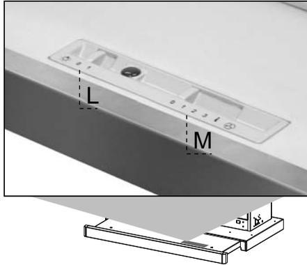
By pulling out the sliding panel it is possible to automatically activate all the hood functions. By simply closing the sliding panel all the functions are switched off.
