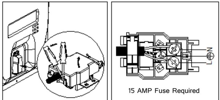
pull open the cover of the terminal board.
