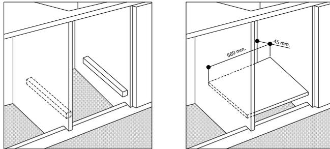
The panels of the adjacent cabinets must be made of heat-resistant material .In particular ,cabinets with a veneer exterior must be assembled with glues which can withstand temperatures of up to 100°C .
