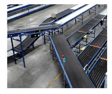
End pulleys are 2-1/2" diameter to **reduce gaps** between units for small product transportation. A belt-low configuration eliminates the guard rail on floor-mounted conveyors and reduces guard rail requirements for overhead units. The CRUZ®channel seamlessly matches other TGW Systems CRUZ®channel technologies - NBC™ XenoPRESSURE®, or IntelliROL®.
