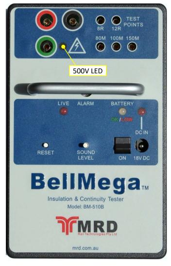
Any Leakage Resistance less than 110M $\Omega$  will trip the unit; the high voltage drop – 371V @ 0.909M $\Omega$  is not relevant. The detection of the Leakage Resistance is a function of the regulated high-voltage supply (1%) and the calibrated internal resistance.
