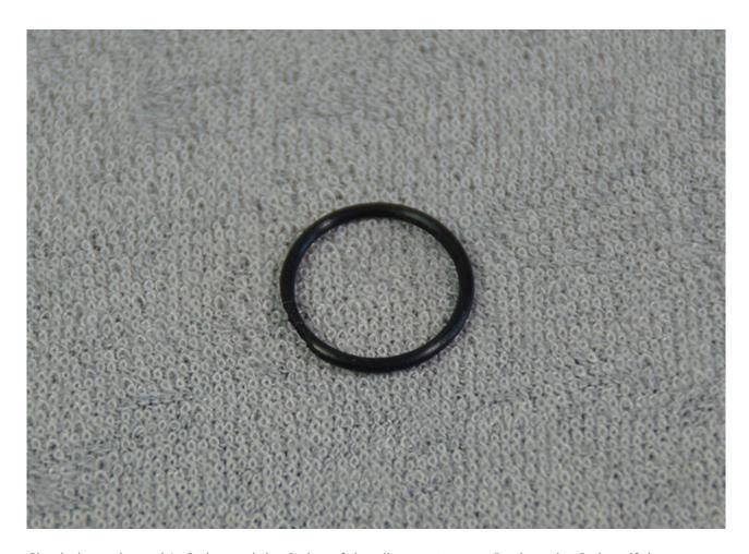
Check the spring unit's O-ring and the O-ring of the alignment screw. Replace the O-rings if they are worn out.
