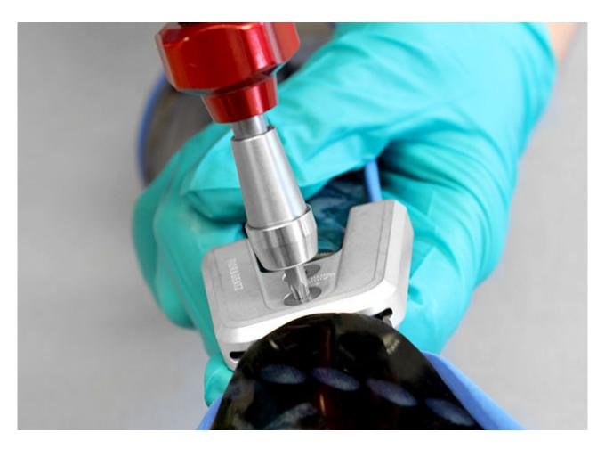
Follow the online tutorial for the joint assembly of system ankle joints with plug + go modularity in order to reassemble the system joint.
