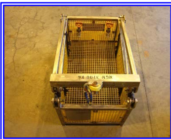
Ubas D with parking receptacles and strapping plates for EFL/OFL.
