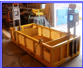
Ubas G with 3 compartments for combined EFL/OFL and HFL deployment / installation.
