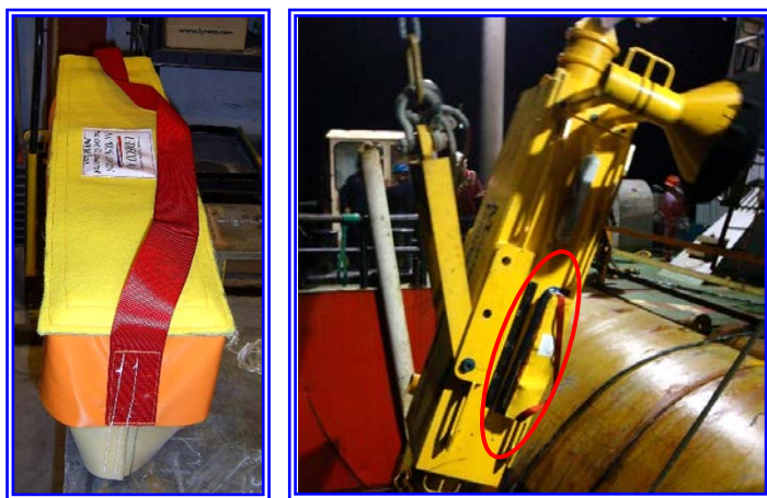
ROV Removable Electrical Connector Block debris on Subsea UTA (FUTA) – Gulf Of Mexico The FUTA was landed onto a pre-installed two segment Umat (temporary mat type)
