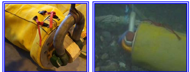
Ucap nose with swing clamp during test and when on seabed / in rock dump.
