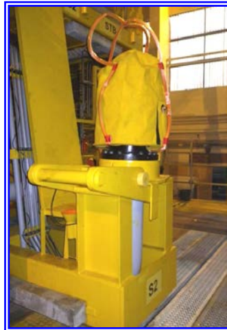
Vertical Ucap installed onto dummy inboard connector and onto actual inboard connector cap.
