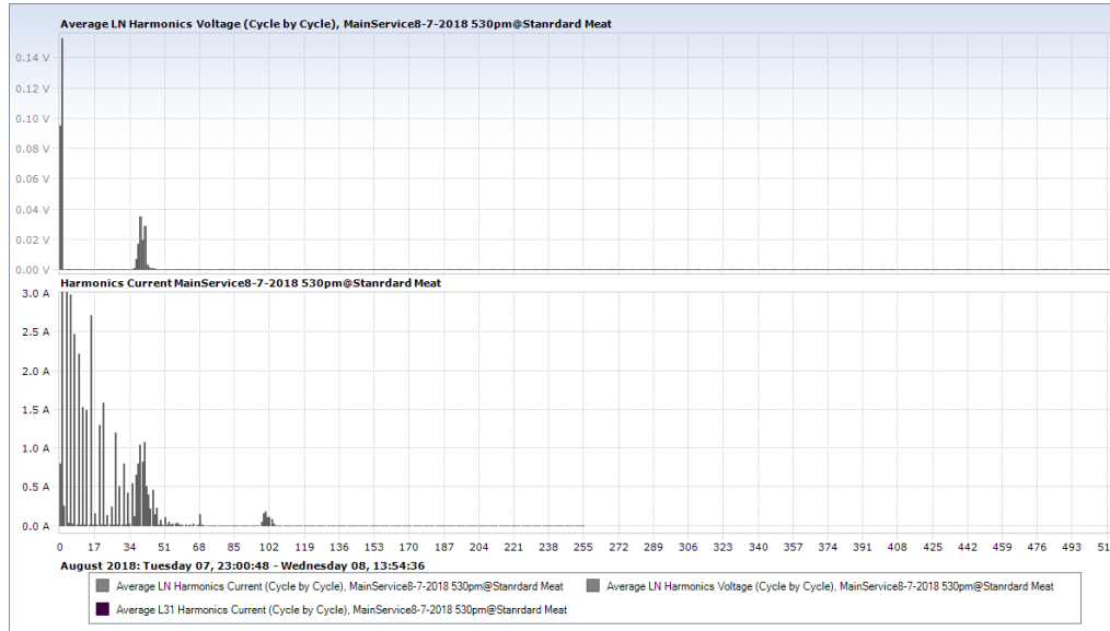
Figure 15 Neutral Harmonics before installation of EP Units
