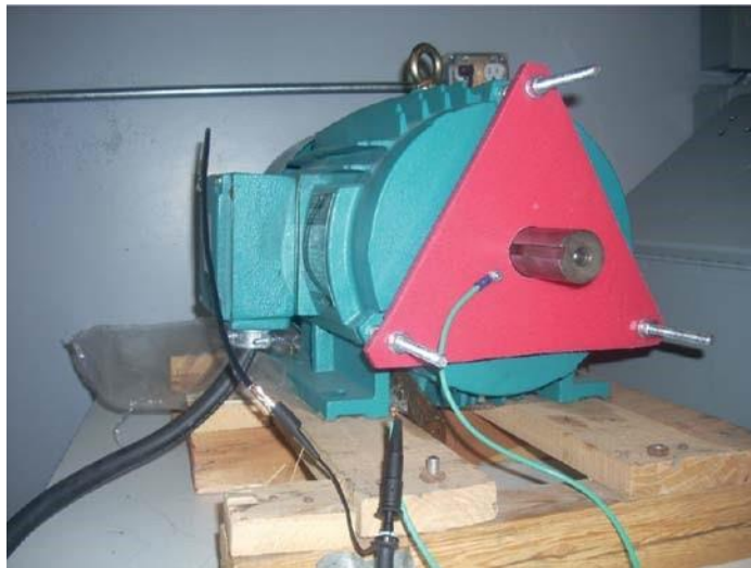
Figure 1: Test setup to measuring bearing currents. Brush connected at the shaft with green wire out, and black wire out from motor casing.
