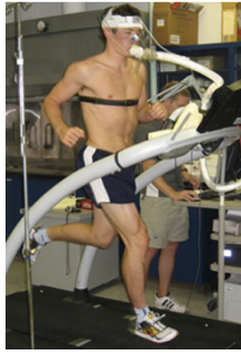
Figure 1: Example of a gold standard VO 2 max measurement using a treadmill, a metabolic cart, a chest strap HR monitor and a gas mask.
