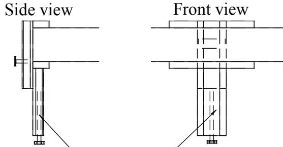
Ensure clamping plate is able to move into the horizontal position before tightening.
