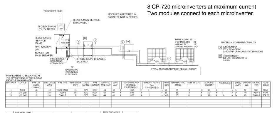
Note: While the CP-720 includes an integrated ground, Chilicon Power recommends installing an equipment ground line to meet the requirements of most AHJs.
