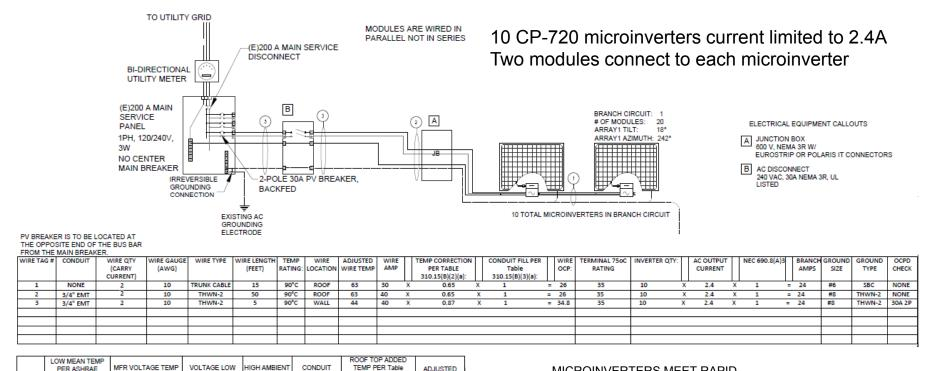
MICROINVERTERS MEET RAPID SHUTDOWN REQUIREMENTS PER NEC 2017 SECTION 690.12
