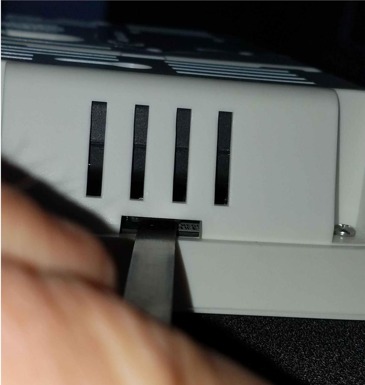
4. Using tweezers, gently pull out the SD card by its sides as shown in the picture below:
