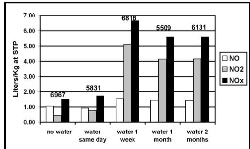
Fig. 2. Nitrogen oxides production for emulsion shot in steel pipe following exposure to water for up to two months. Numbers above bars are detonation velocity in m/s (Rowland, Mainiero and Hurd [5])
