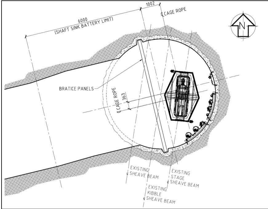
Figure 8 K2 shaft internal layout (note 60/40 split and 2 guide ropes only for cage)
