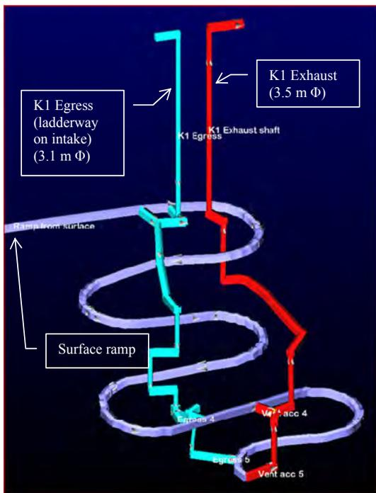
Figure 4 Existing K1 simple whole-of-mine series ventilation circuit
