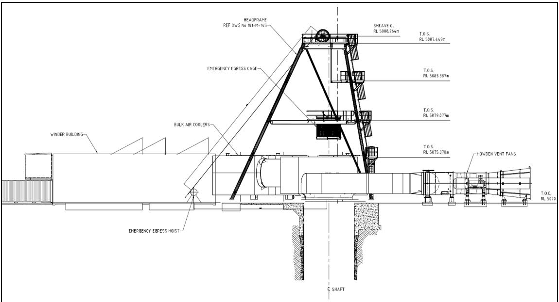
Figure 12 K2 shaft surface (elevation)
