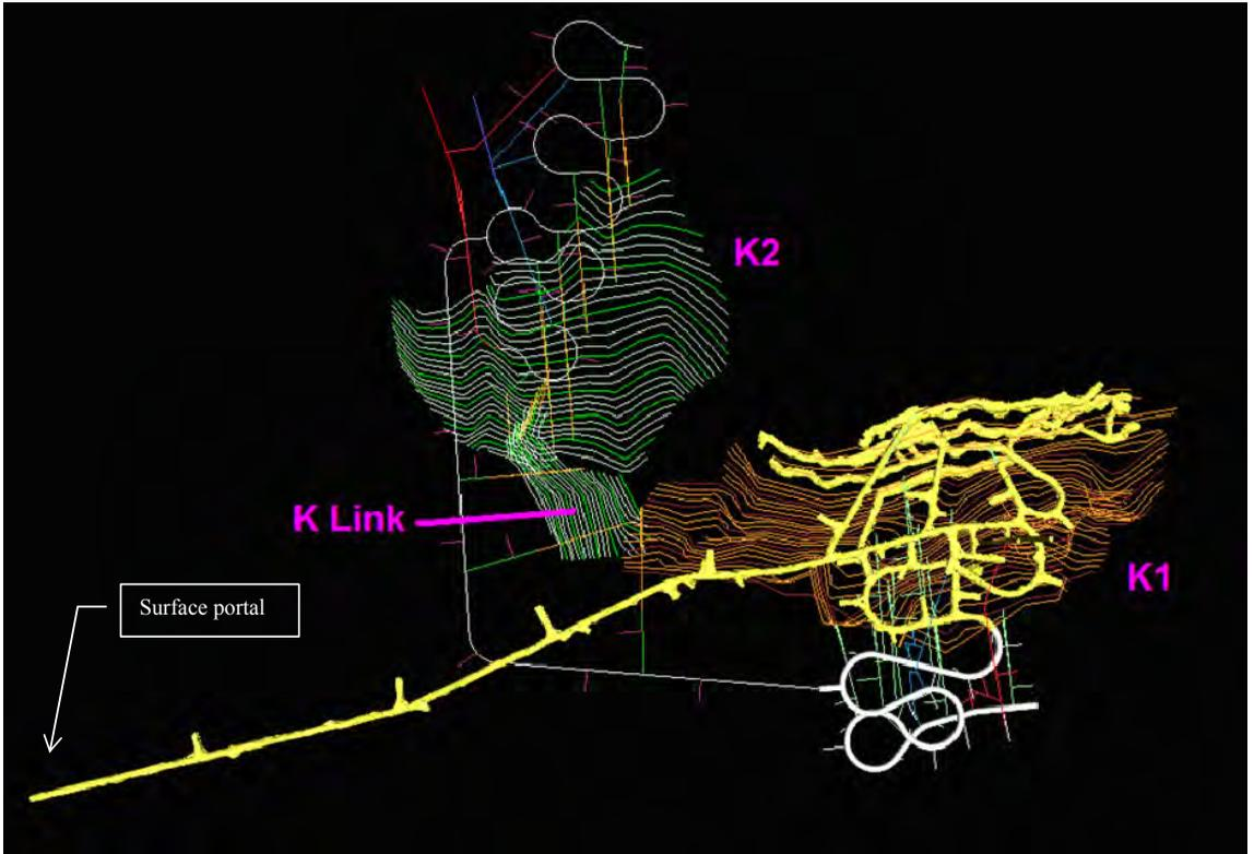
Figure 2 Plan view of K1 (existing), K2 and K Link (under development) orebodies
