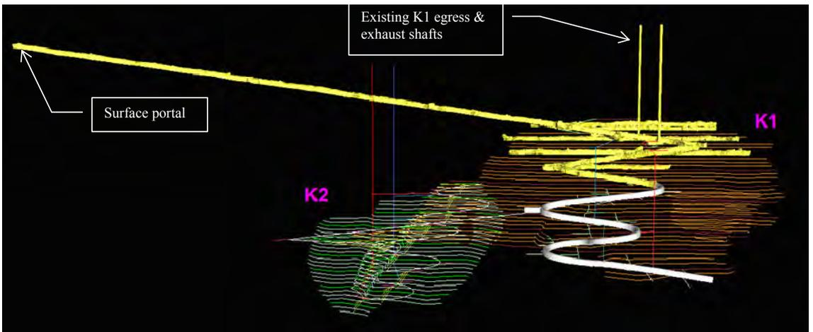
Figure 3 Section view of K1 (existing) and K2 (under development) orebodies. K Link is mid-way between K1 and K2
