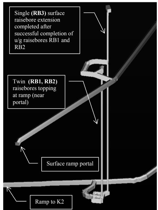
Figure 5 Twin raisebores for initial K2 development (and longer-term ventilation of K Link production)
