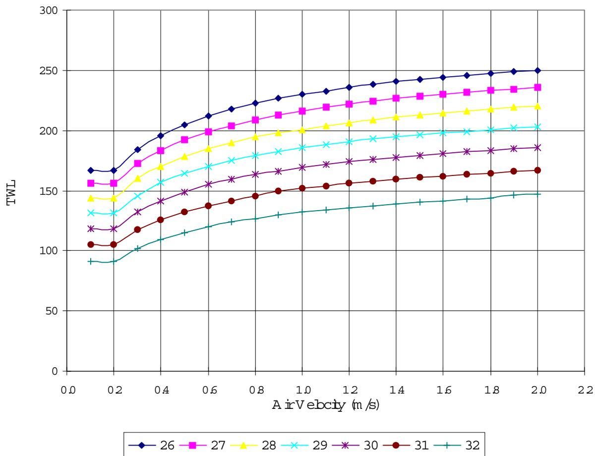
**Figure 7 Reduction in airflow required in underground workshop after introduction of refrigerated air**
