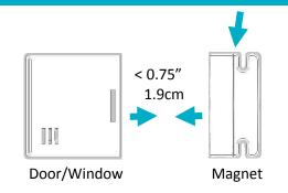
Install the Magnet in the proper orientation using 2-sided tape or screws. The Magnet must be within 0.75" (1.9 cm) of the Door/Window Sensor.
