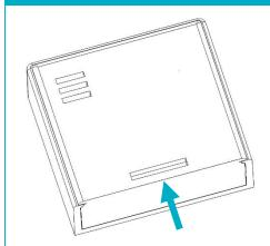
Once you have installed the bottom housing and confirmed the device is communicating, insert the Door/Window Sensor's top housing as shown above
