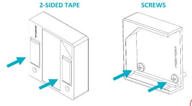
**Notes:** Installation on metal can reduce transmission range. Ensure that the device is installed in a dry location away from running water, excessive moisture, and rain.
