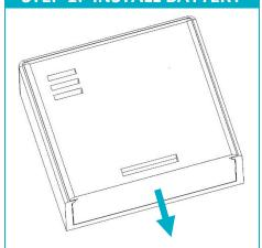
Slide open the Door/Window Sensor's top housing. Pull the plastic tab from the CR2032 battery in the housing top as shown below.
