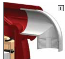
Down outlet and connection to drainage pipe
