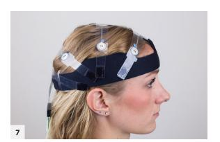
Proper sensor strip and neoprene head strap placement is crucial in order to acquire high quality data.
