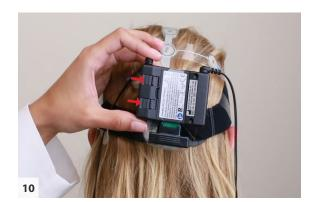
Reattach the Headset door and lock it in place by sliding the tabs toward the center of the Headset. Connect the 3-pin linked mastoid cable, and optional 2-pin leads, to the Headset.
