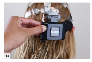
Turn on the Headset. Allow Headset and Receiver to pair, as indicated by a solid light on both devices.
