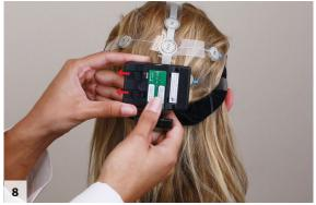
With the Headset upside down (USB port facing up), unlock and remove the door by sliding the tabs away from the center.
