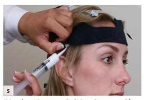
Using the syringe, part the hair at the temporal foam sites and add synapse cream to the foam sensors. Once all temporal sites have been filled, attach the remaining strip tabs to the neoprene head strap.
