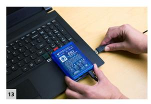
Attach the Bluetooth Receiver (ESU) to the USB port on the computer.
