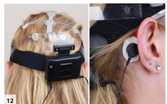
12 Attach the 3-pin linked mastoid cable to the mastoid electrodes.
