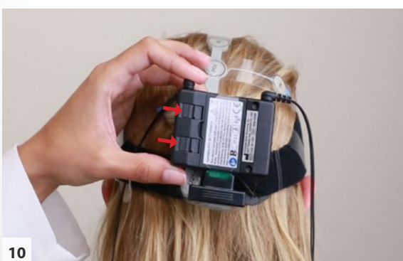
10 Reattach the device door and lock it in place by sliding the tabs toward the center of the device. Connect the 3-pin linked mastoid cable, and optional 2-pin leads, to the device.
