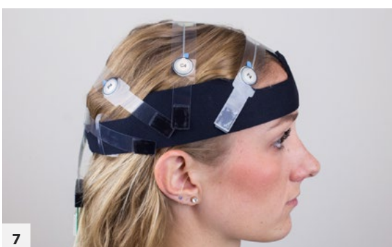
7 Proper head strip and strap placement is crucial in order to acquire high quality data.
