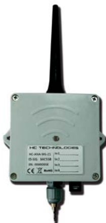
HC-ANA-SIG with integrated temperature, moisture and illumination sensors
