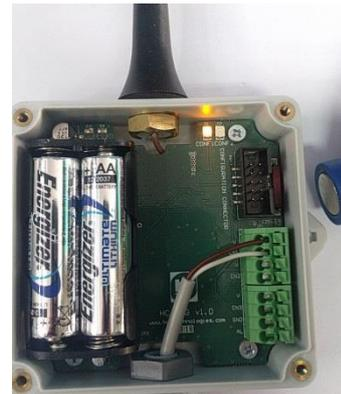
**State 2:** Magnet placed for more than 1 second and less than 3 seconds close to the mark. The CONF1 led (yellow) will light twice. In this case, a configuration packet will be sent (contains the internal configuration of the device). (Contact HC Technologies to receive the format and description of the packet).
