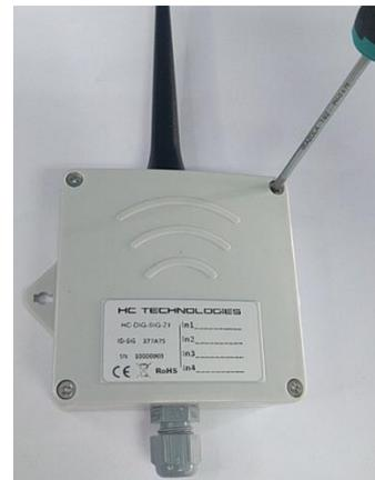
**STEP 2:** Connection of sensors. This device allows the connection of analog sensors (and 1 extra digital sensor) through 2 wire cables per sensor. The analog sensors (resistance type) should be connected to V and CnX input. The input cables are passed through the cable gland to guarantee tightness. For information on how to connect other kind of sensors to the device please contact HC Technologies.
