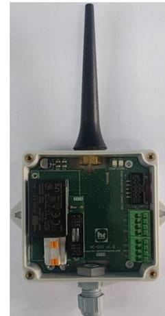
The internal AC power system has been designed so that you can not have contact with the AC signals at any time. In addition, a 5x20 mm 240V 100mA fuse protected by a plastic cover is used. In the event of a short circuit or any other problem, to replace the fuse, remove the plastic cover, insert the new fuse in the cover and reconnect the plastic cover to the fuse holder.
